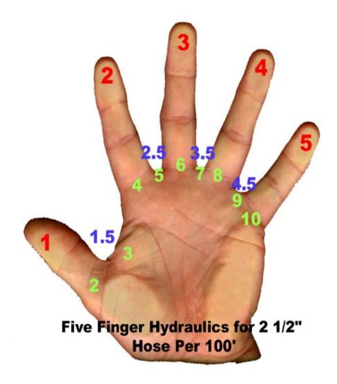
The base numbers are coefficients used as multipliers to determine friction loss per 100 ft of  $2\frac{1}{2}$  hose. To complete the process remember to add the lengths of hose. This will give you total friction loss for you calculation. This information is put in the engine pressure equation
