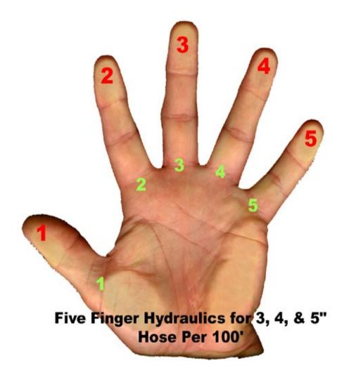
To determine friction loss in 5`` hose calculate fingertip times finger base as in the 3`` system and then divide your answer by 12. Example 5`` hose flowing 1000 GPM, tip of 10 times the base of 10, divided by 12 equals 8# per 100 ft. For higher flows simply count on both hands.
